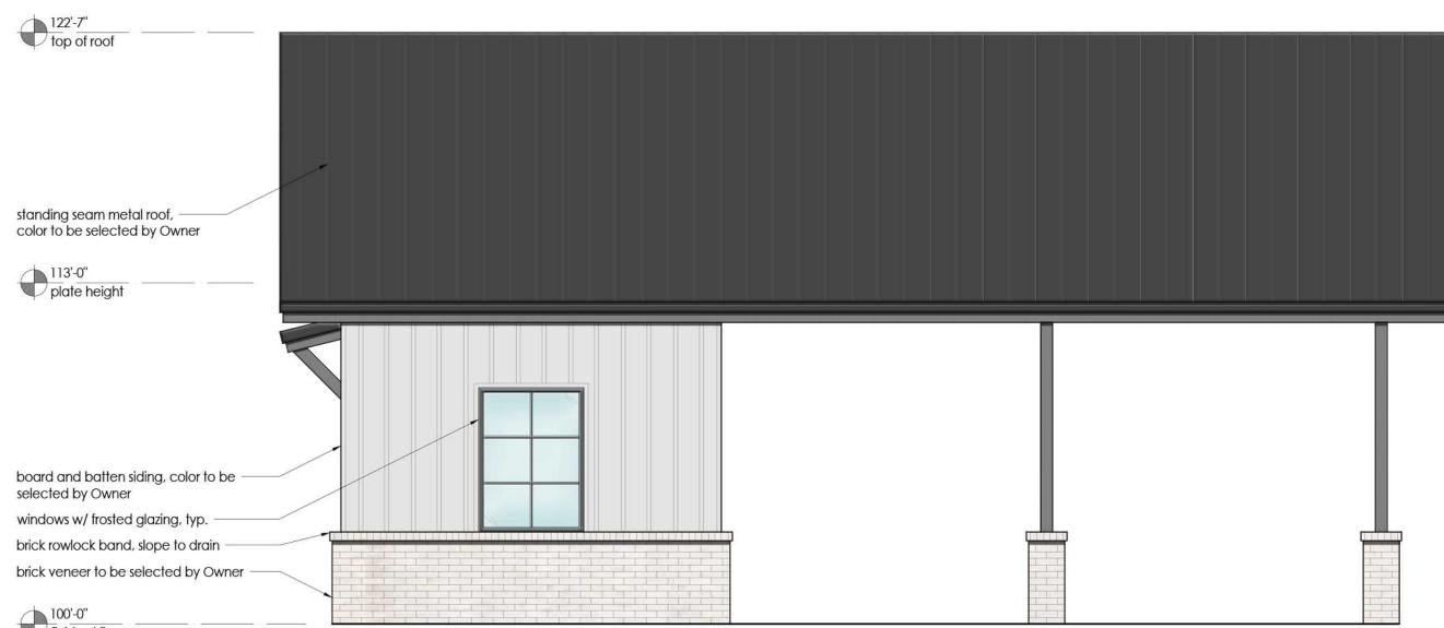
windows w/ frosted glazing, typ. brick rowlock band, slope to drain -
